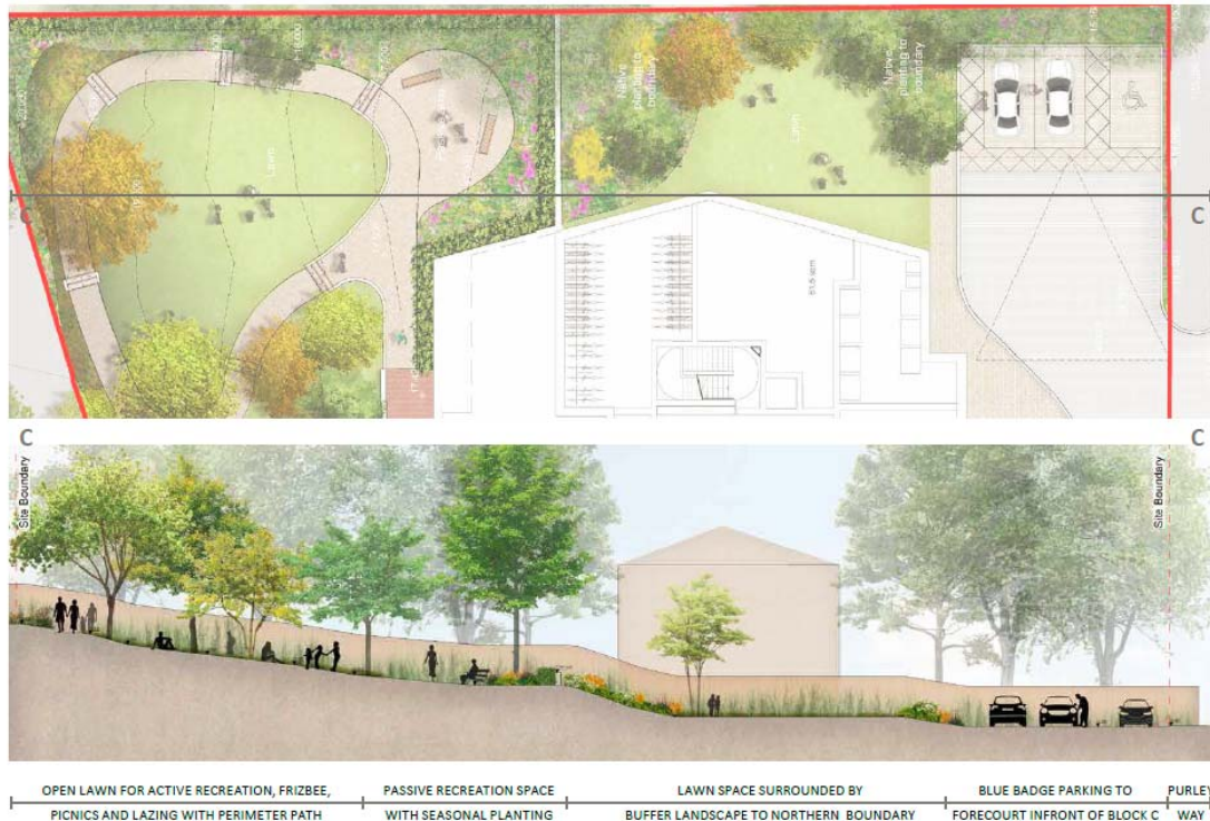
Figure 8: Proposed land levels at the rear of Block C and adjacent to 920 Purley Way
