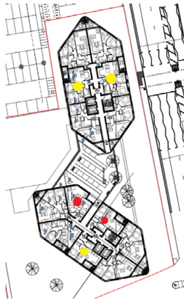
Fig 8 - Plan indicated the single aspect units which are either not north facing (yellow dot) or which are north facing (red dot) on typical floorplan.
